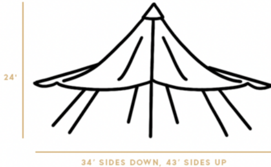
Figure 3. Graphical representation of Sami Tent with Dimensions. The sides of the tent are held up and there are no walls.
