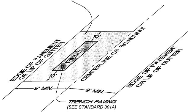
NOTE: \* IF THERE ARE 2 OR MORE TRENCHES WITHIN 300 FEET OF THE STREET, THE SLURRY SEAL SHALL APPLY CONTINUOUSLY TO COVER ALL TRENCHES.
