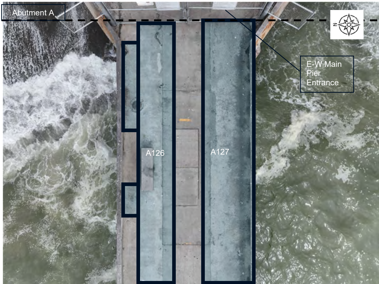
Figure A.2-43 Delaminated Areas around Abutment 1-A
