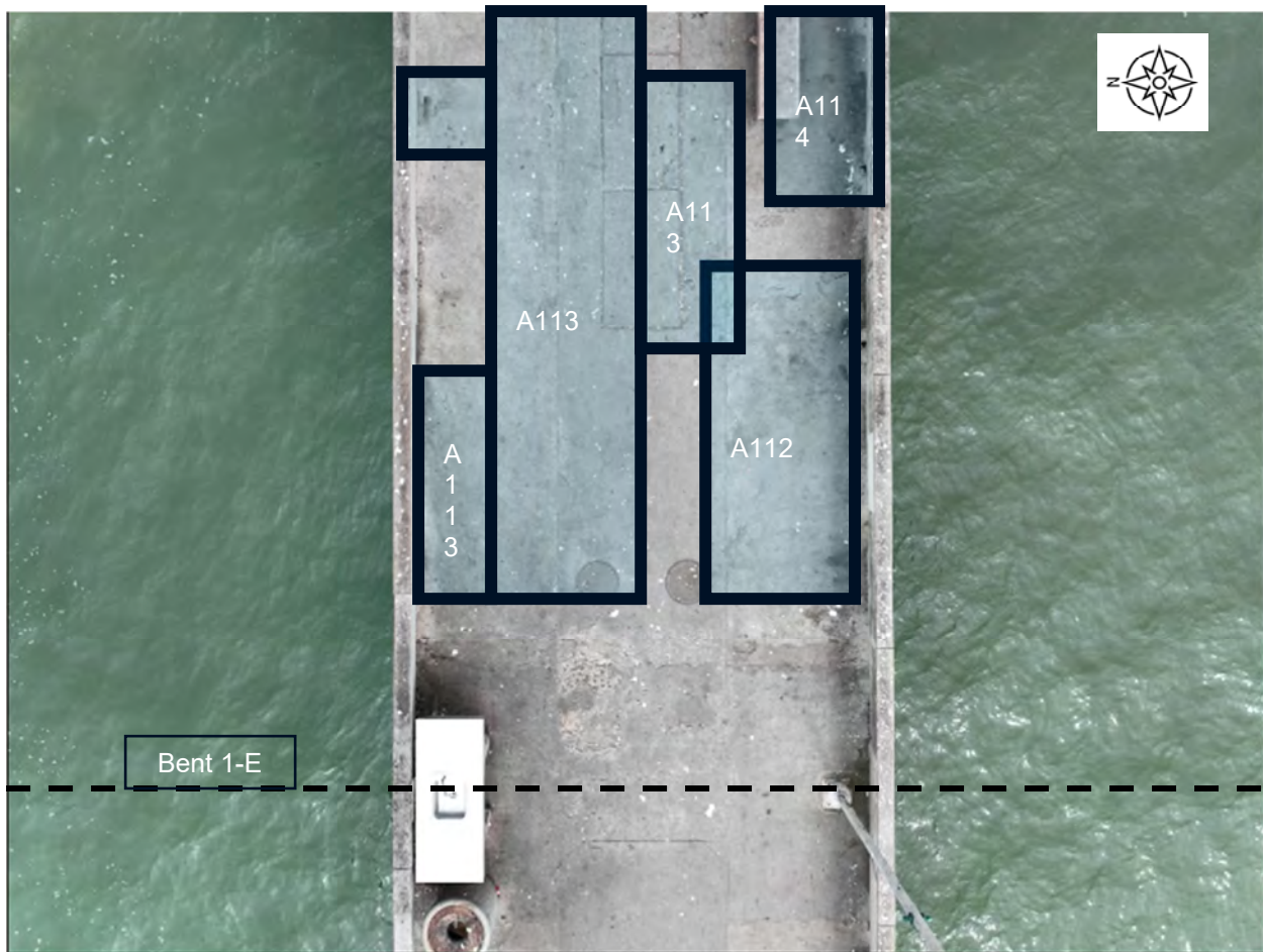
Figure A.2-37 Delaminated Areas between Bent 1-E and Bent 1-D – E-W Main Pier
