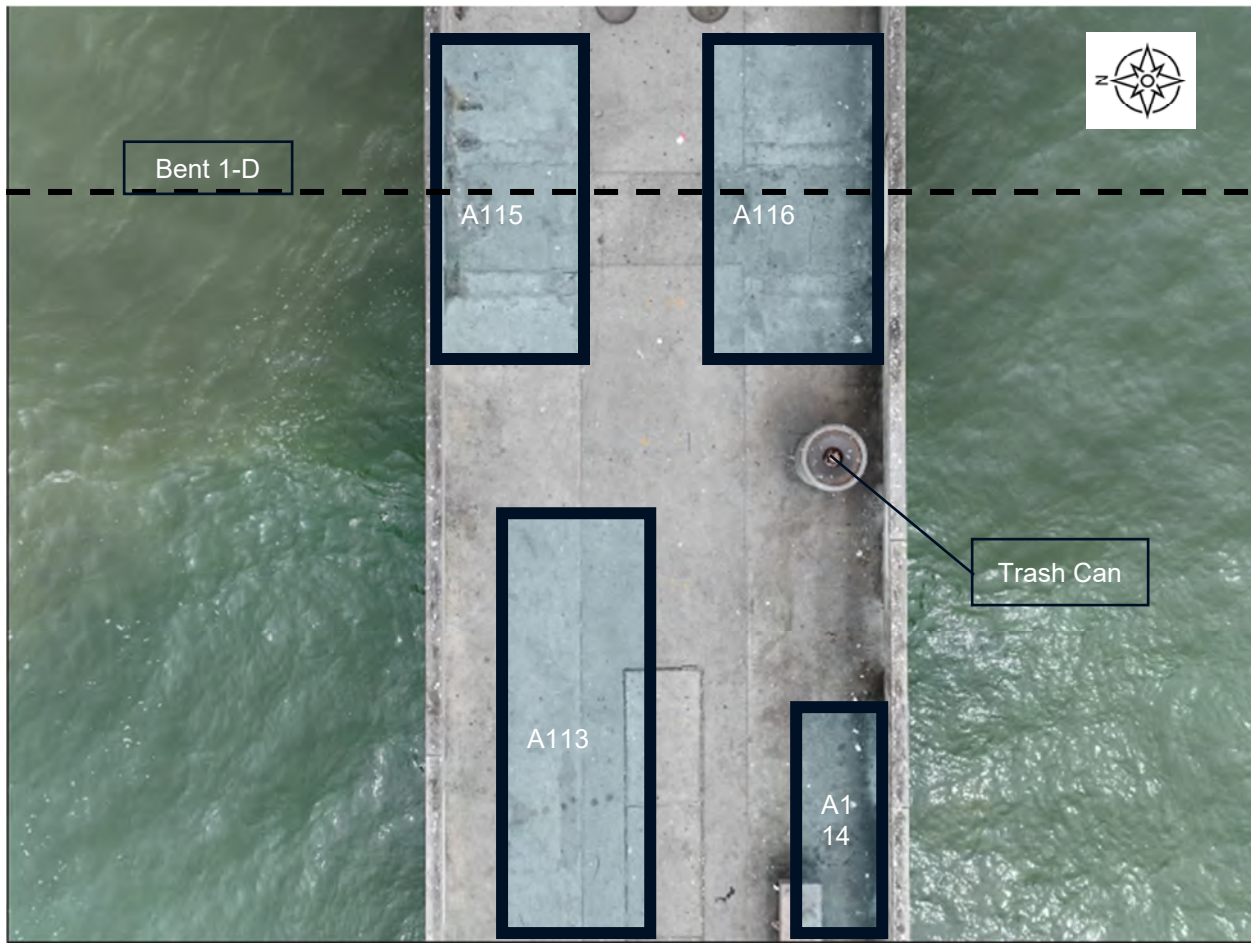
Figure A.2-38 Delaminated Areas around Bent 1-D – E-W Main Pier
