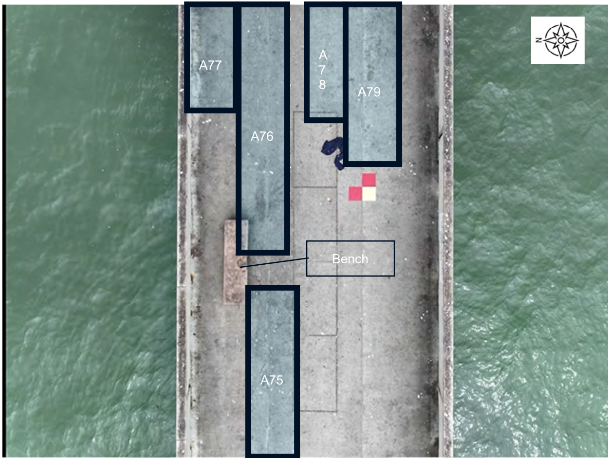
Figure A.2-24 Delaminated Areas between Bent 1-L and Bent 1-K – E-W Main Pier
