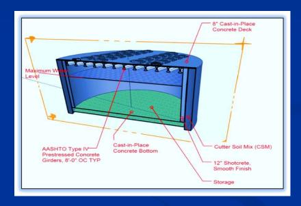
Based on the information available at the time, a cylindrical-shaped basin was thought to have the greatest strength and be the easiest to construct.
