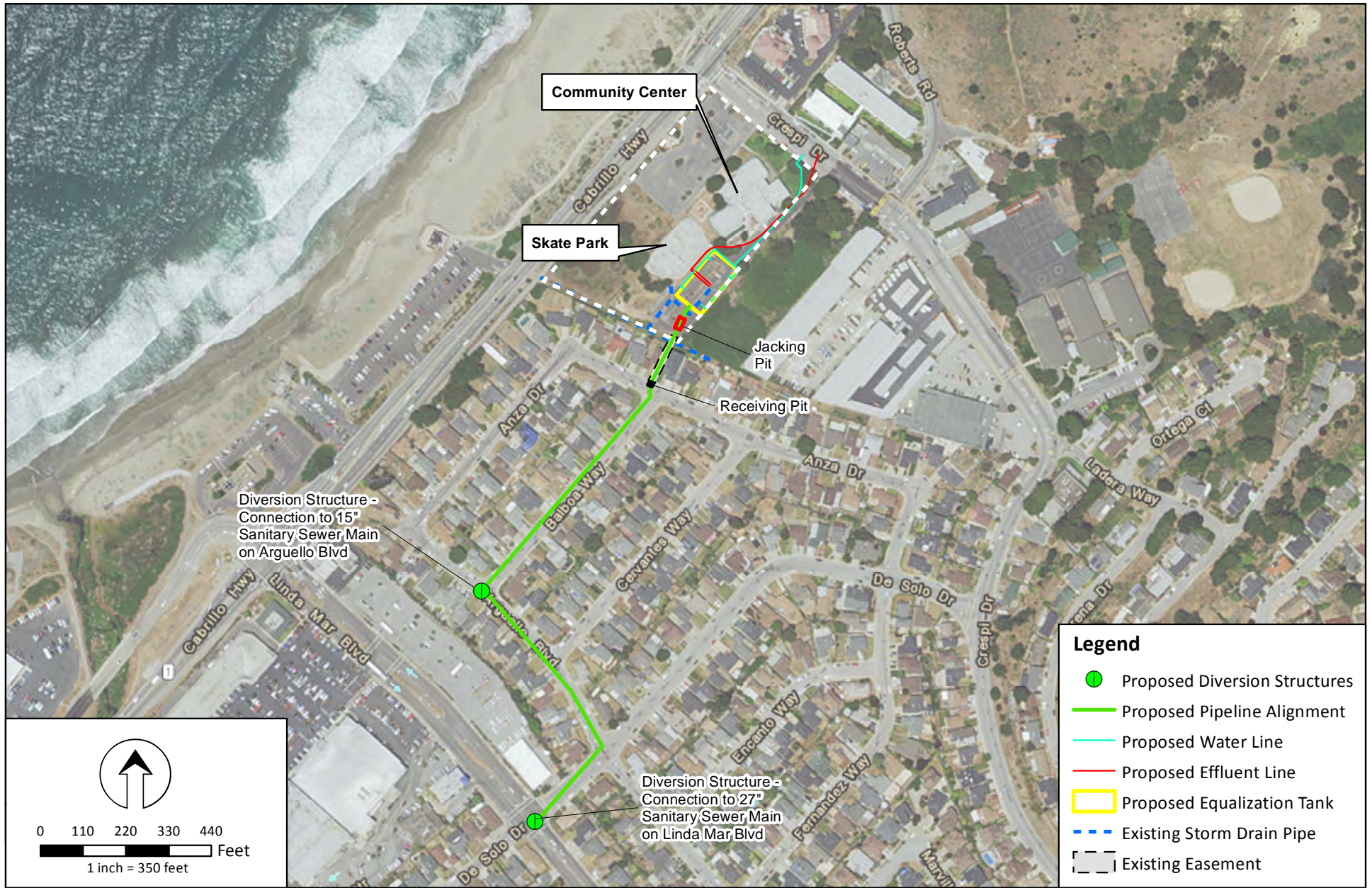
Figure 4 Proposed Locations of the Diversion Structure, Jacking Pit, Receiving Pit, Influent Pipeline, and Effluent Pipeline
