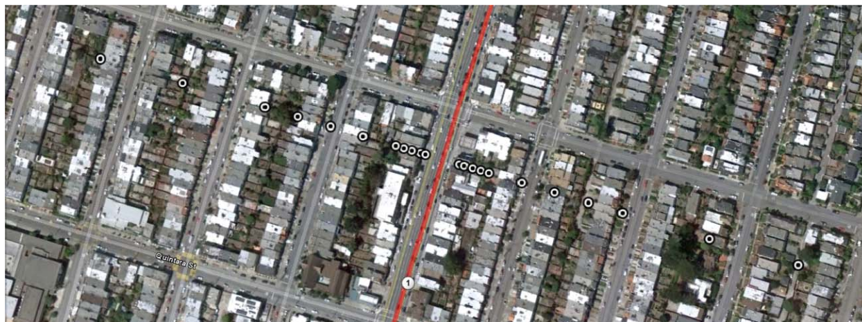
Figure 10. Receptor locations (shown as white circles) to the west and east of a roadway link (shown as a red line). Receptor distances were taken from the edge of the roadway.
