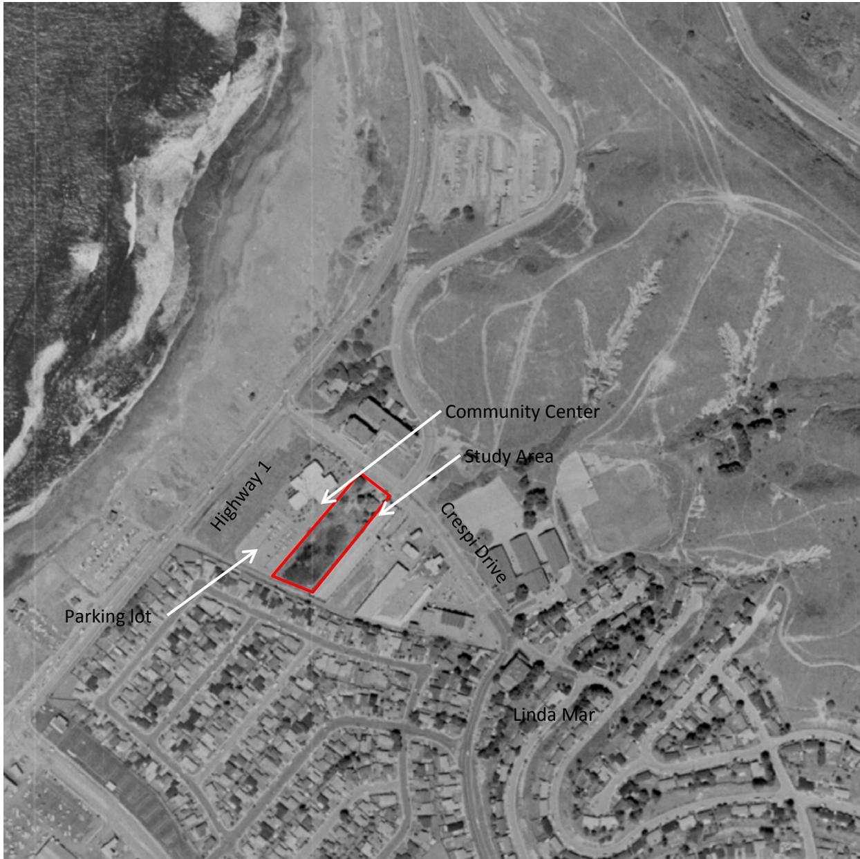
**Figure 5.** Aerial photograph, 1980. Dark vegetation within study area suggests wetlands forming following construction of parking lot, which may have limited lateral movement of shallow groundwater.
