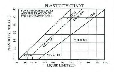
Reference: ASTM D 2487-98, Standard Classification of Soils for Engineering Purposes (Unified Soil Classification System).
