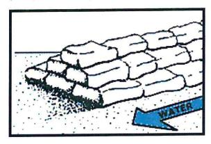
Figure D. When you don't have time to build a sandbag barrier, use a temporary levee to raise low areas. Prepare ahead by buying 20-foot wide sheets of plastic (6-10 mil. thickness). Lay out the length you need and place sand, dirt or gravel on the half facing your property. Fold over the other half and place a solid row of sandbags on the edge of the plastic to anchor the top edge of the plastic sheet.
