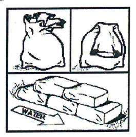
Figure C. Place a line of bags with the folded side up, with folded edges facing the direction of the water flow. Stomp each bag into place. Like you would with bricks, stagger the next layer of bags over the tied top of the bags underneath. Stomp each layer of bags. To give the structure stability, the base should be 1.5 times wider than the height. (Example: 6 ft. wide by 4 ft. high)
