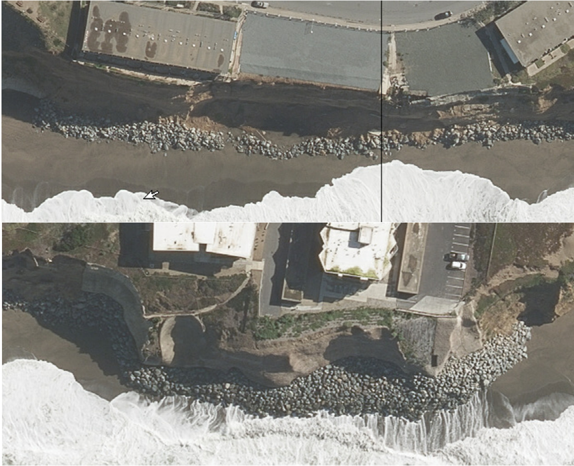
Figure 11 Bluff toe armorment and erosion at Esplanade blufftop apartments (top) Bluff toe and face armorment at The Bluffs apartments (bottom)
