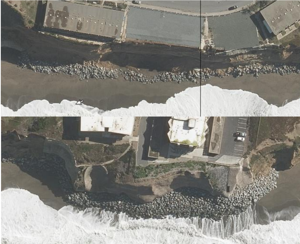
Figure 11 Bluff toe armoring and erosion at Esplanade blufftop apartments (top) Bluff toe and face armoring at The Bluffs apartments (bottom)
